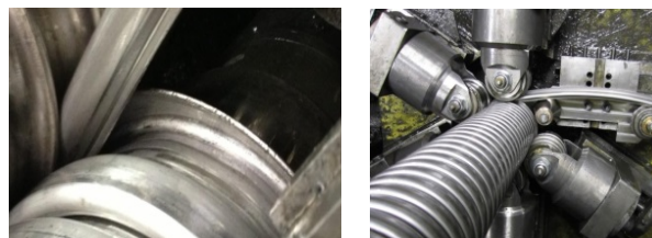
Figure 6. Manufacture process of carcass layer [41]
