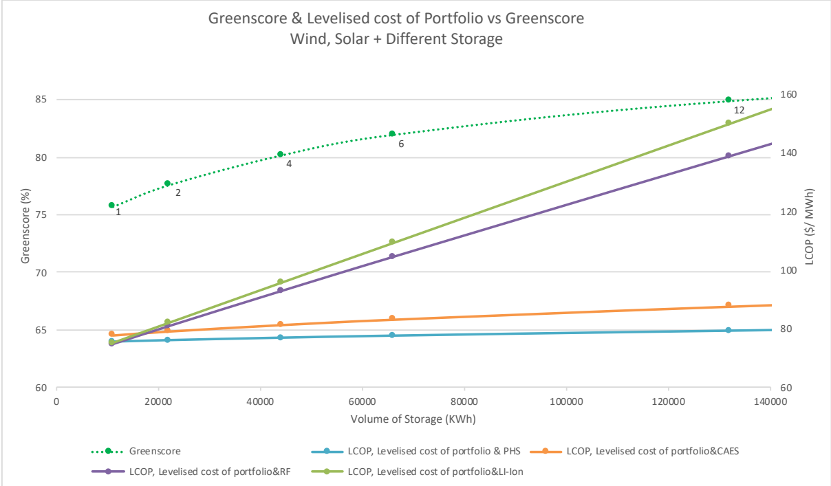
Figure 39: Green score & levelised cost of portfolio vs green score of wind, solar PV and different storage technologies
