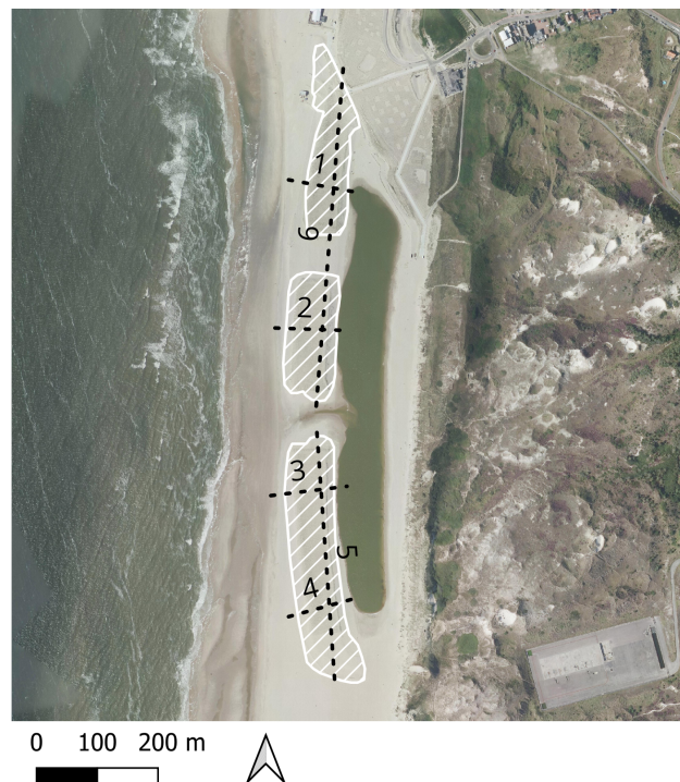
Figure 5.8: The six locations where the cross sections are taken. Other cross sections are taken through the channel from north to south and through the opening in the north, from north to south as well.
