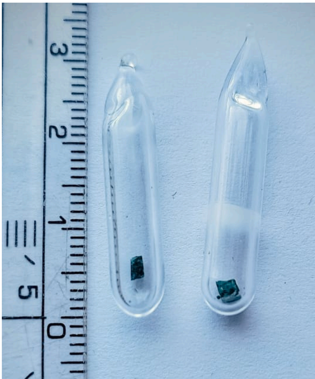
Fig. 1. Millimeter sized crystals of NaI:0.2%Sm 2+ (left) and NaI:0.2%Tl + ,0.2%Sm 2+ (right) crystals sealed in silica ampoules.
