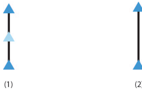
Figure 3.7: The simplification of straight line segments during the reading process. When passing over a "F" char no new point is stored nor a new edge if the next char is also an "F". The location of the turtle does get updated however. If the next "F" char is not followed by another "F" char, the point and edge are stored. (1) the location updates of the turtle, (2) the stored edge and points.
