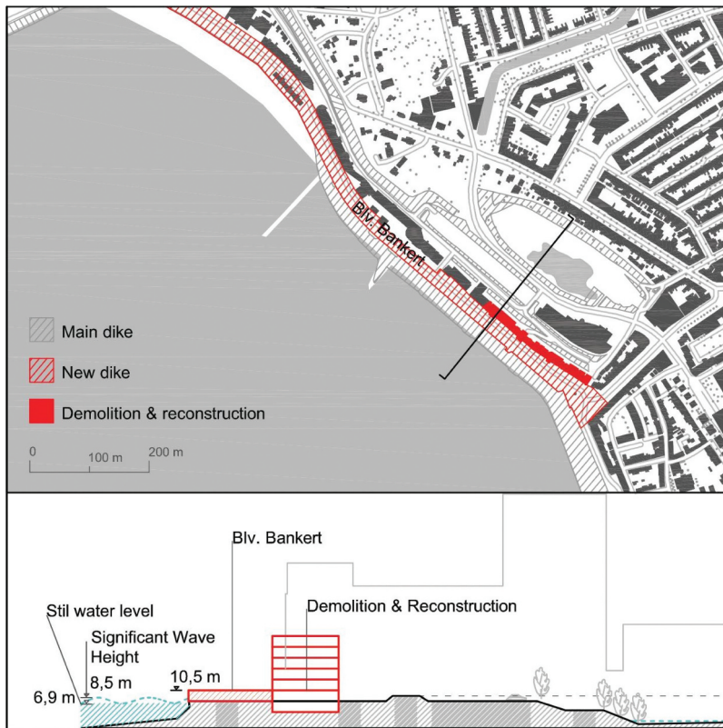
Figure 3. Spatial design strategy: the Vlissing Model; plan and prototypical section (elaboration: A. Bortolotti).
