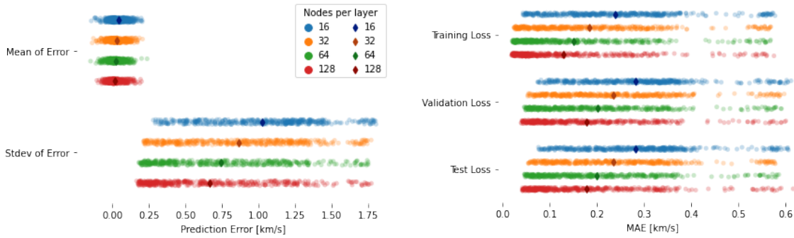
(a) The training loss, validation loss and test loss for the ANNs containing different numbers of nodes per layer. The selected loss function is the MAE. (b) The mean and the standard deviation of the prediction error of the ANNs for different numbers of nodes per layer.
