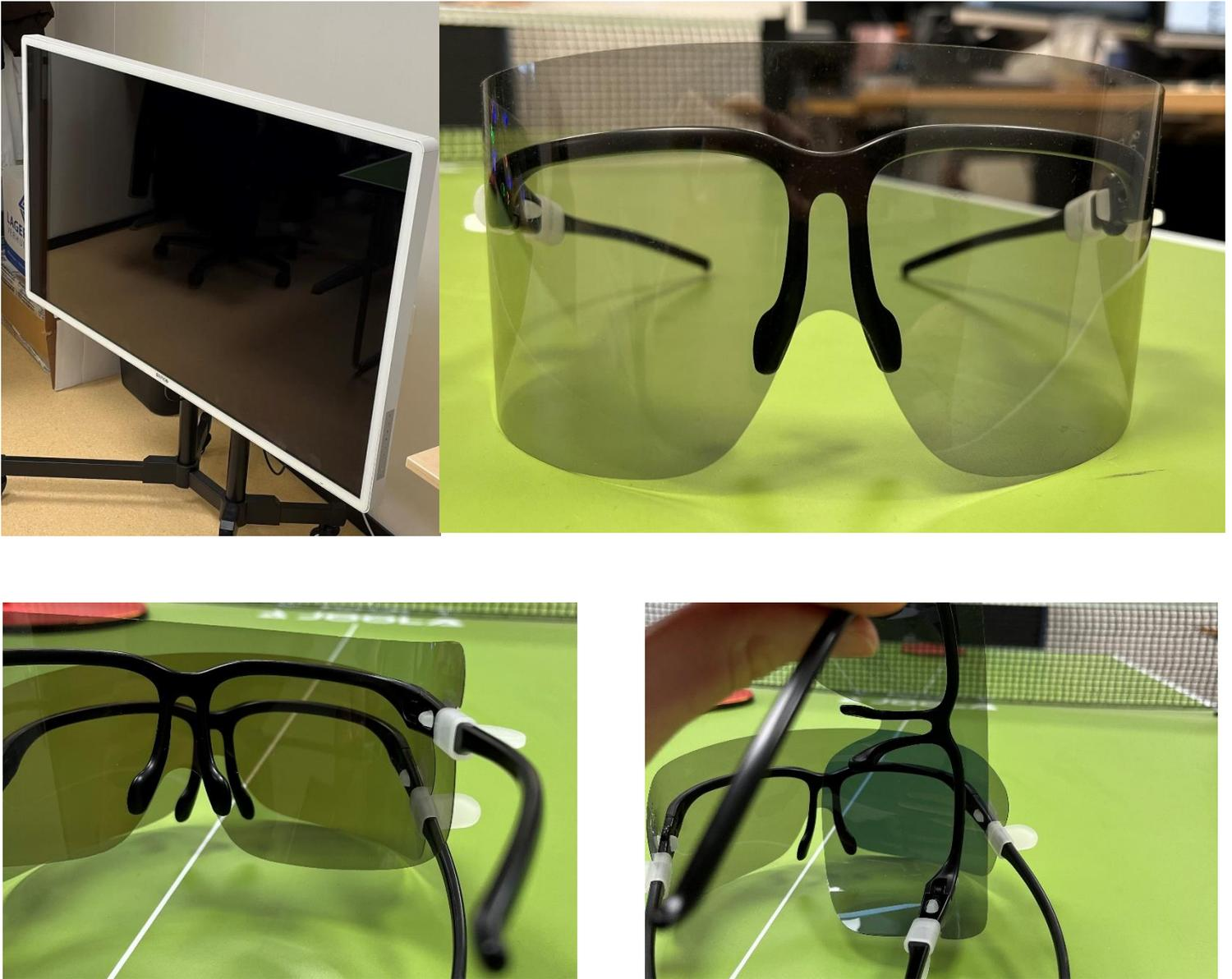
Figure 3. Images of the stereoscopic display and 3D polarized glasses
