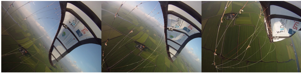
Figure B.3: Collapse of the entire wing during reel-in, from the perspective of the wing tip video camera.
