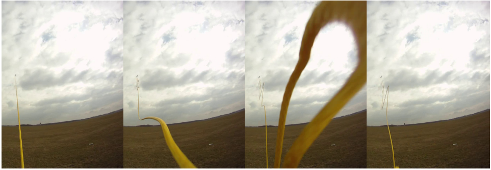
Figure B.5: Backlash of the tether after rupture at the kite end. Video stills at 100 ms intervals.
