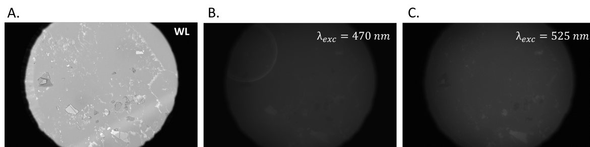
Figure 67: hBN flakes mechanically exfoliated on a Blu-ray disk: A. White light image. B. Fluorescence microscopy taken with the 470 nm filter set with an exposure time of 119 ms and an analog gain of 19. C. Fluorescence microscopy taken with the 525 nm filter set with an exposure time of 1 s and an analog gain of 38.
