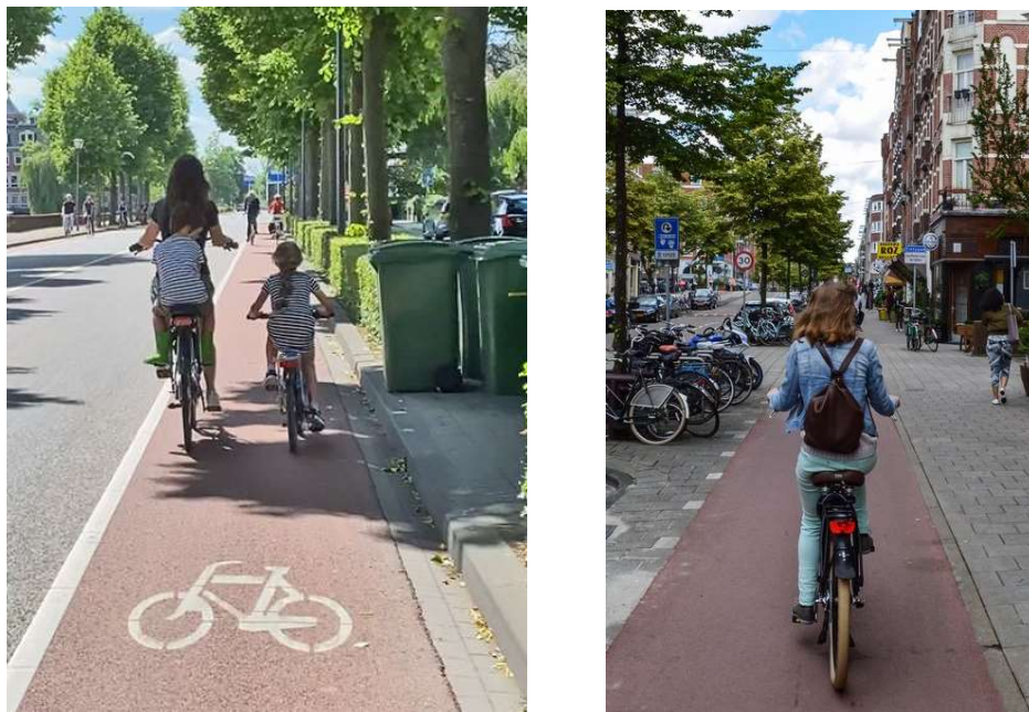
FIGURE 3 – DIFFERENCE BETWEEN AN ON-ROAD CYCLE LANE (LEFT) (WAGENBUUR, 2020) AND A PROTECTED CYCLE TRACK (RIGHT) (ROBERTS, 2018)
