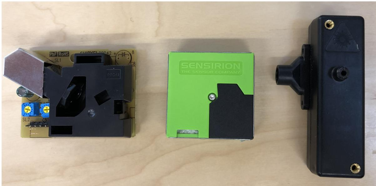
Figure C.2: From left to right: Shinyei PPD42NS, Sensirion SPS30 and AlphaSense OPC-R1 PM sensors
