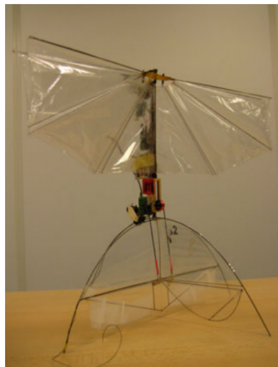
Figure 2.2: 'Standing tail' design of the DelFly [11]
