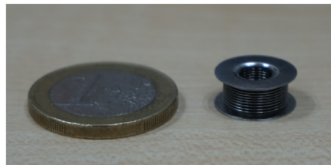
Figure 3.9: Size comparison of the chosen compliant bellow by Guido Mous to a one euro coin [27]
