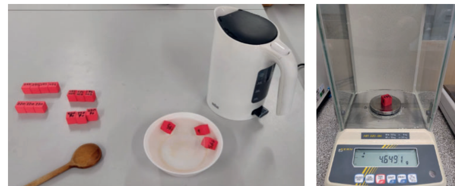
Figure 24: Samples activated in hot water (left) and weighed before and after activation (right).
