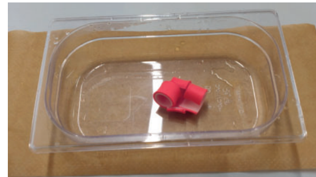
Figure 44: Samples after actuation with hot water poured from the side.
