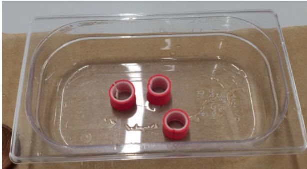
Figure 45: Samples after actuation by hot water dip in.
