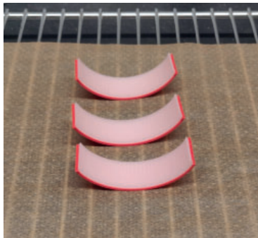
Figure 41: Samples after actuation in the oven without convection.
