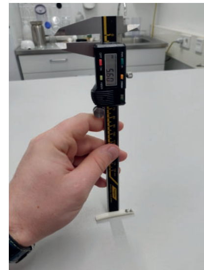
Figure 52: Measuring the gap between the sample and the table with the back of the calipers.
