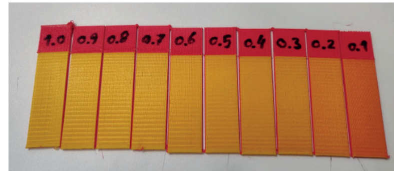
Figure 35: Samples ranging from a 1:1 ratio to a 1:10 ratio before actuation.
