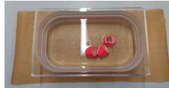
Figure 43: Samples after actuation with hot water poured on top.
