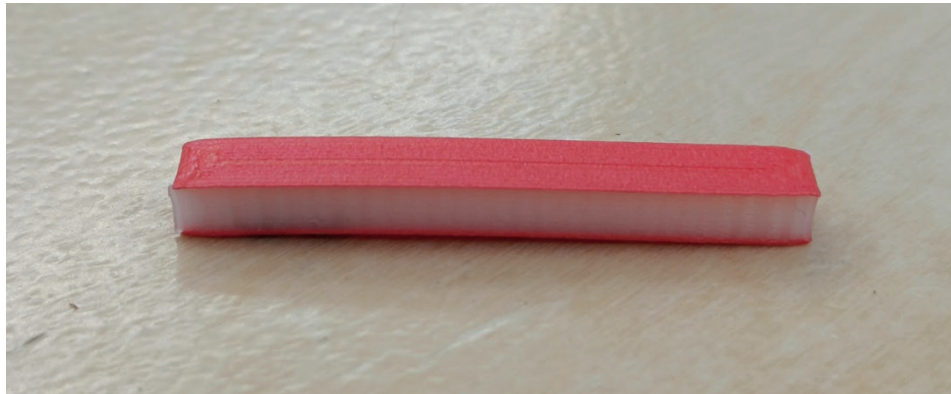
Figure 50: Sandwich structure after actuation in the oven.
