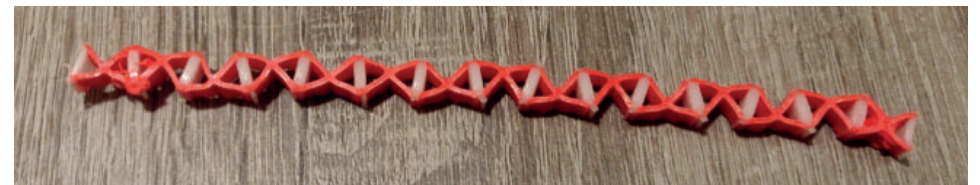
Figure 49: Scissor structure after being actuated in an oven.
