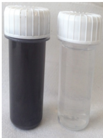
Figure 4.1: Color of the liquids obtained after milling with and without a surfactant.
