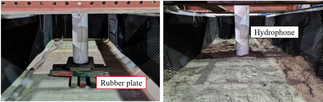
Figure 2: Interior view of the tank showing the rubber plates used to keep the pile position, the soil layer profile, and the hydrophone location.
