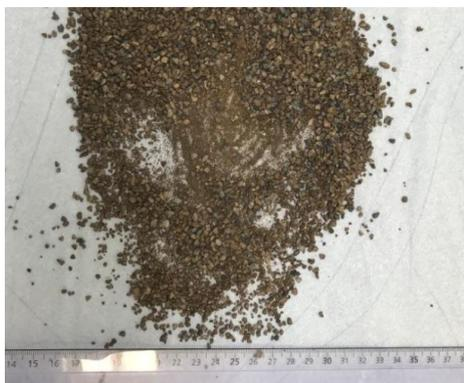
**Figure 5.15:** Catalyst after weeks of experiments
