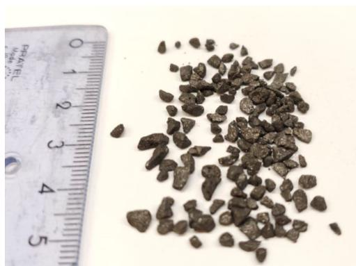
**Figure 5.14:** Fresh catalyst before the experiment
