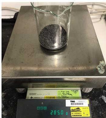
Figure 5.22: Catalyst weight loss
