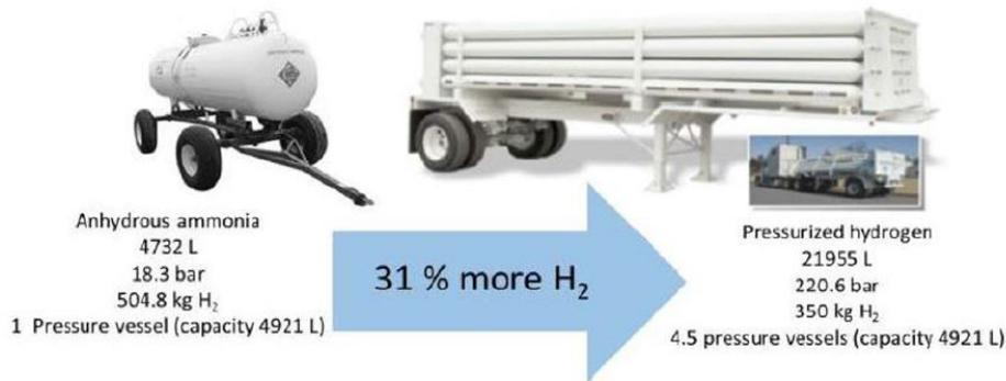
Figure 2.3: Ammonia as a hydrogen carrier distribution [90]
