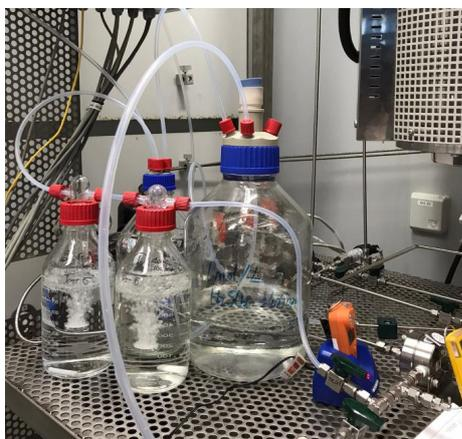
**Figure 4.7:** Sulfuric acid bottles used during the experiments
