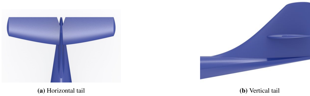
Figure 11.4: Empennage design of the Caty
