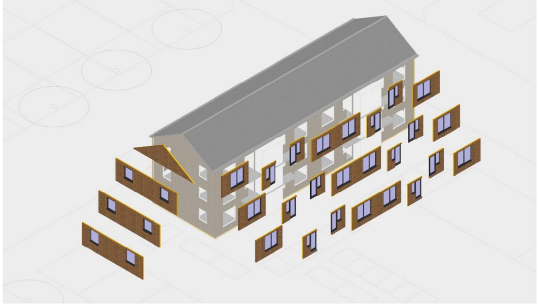
Figure 9.3.2: Facade elements North and East facade, Source: own illustration.
