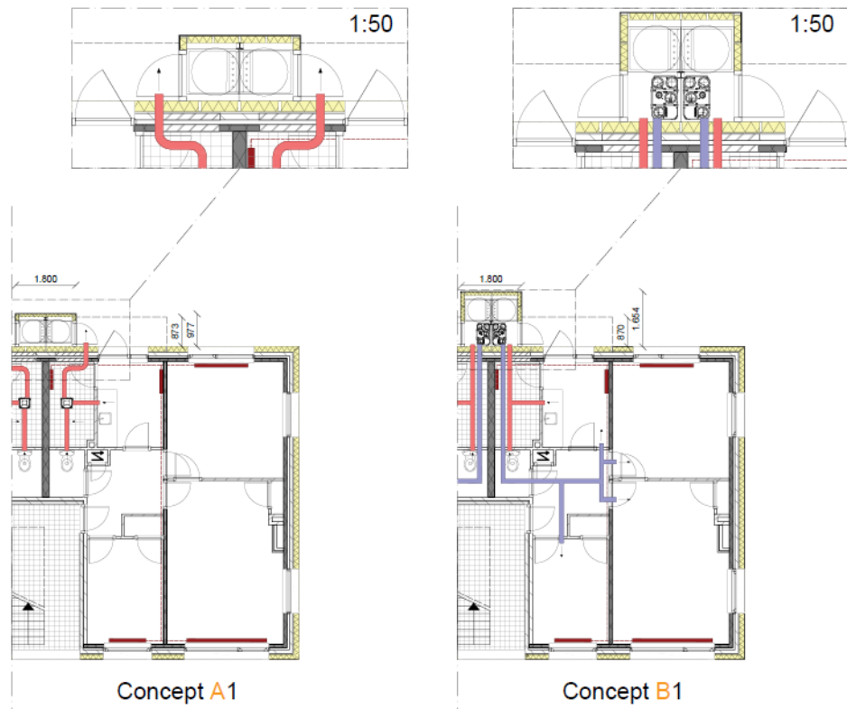
Figure 9.3.5: New floorplan with building services, Source: own illustration.
