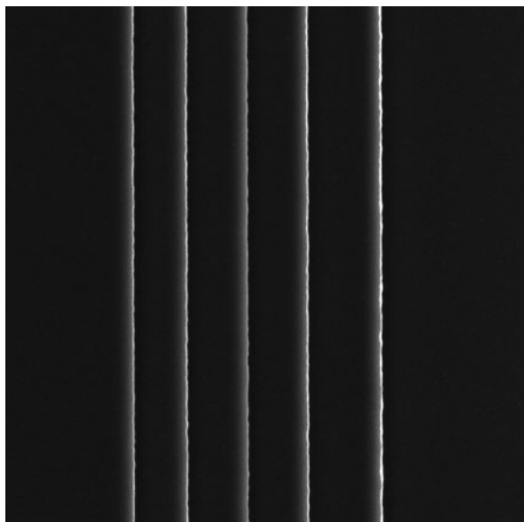
Fig. 20. Top-down SEM image of the steps (only left-side) at 4 keV. FoV = 8.0 \mu\text{m} , taken with the RAITH eLINE Plus SEM.
