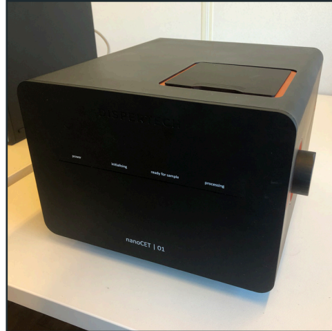
14). The laser inside the NanoCET automatically aligns after clicking a button at Software 1.
