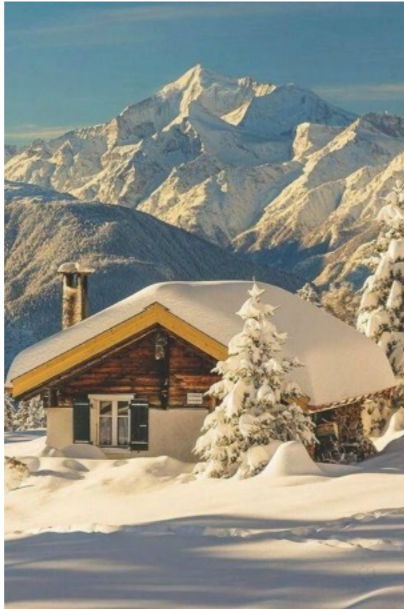
Low pitched roofs - the Alps - Thermal insulation Gentle slope collects layer of snow which insulates the house
