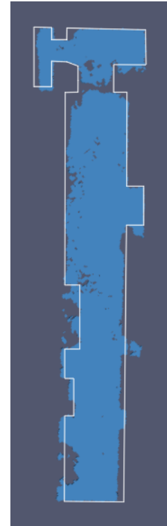
(b) Comparison between identified navigable space and the real world navigable space from a cad!
