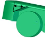
**Figure 2.15:** Illustration of chamfer fill in a wheelhouse (Mavuri and Watkins, 2011)
