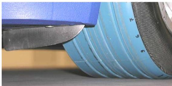
**Figure 5.50:** Wheel spoiler in front of wheel (Dimitriou and Klussmann, 2006)
