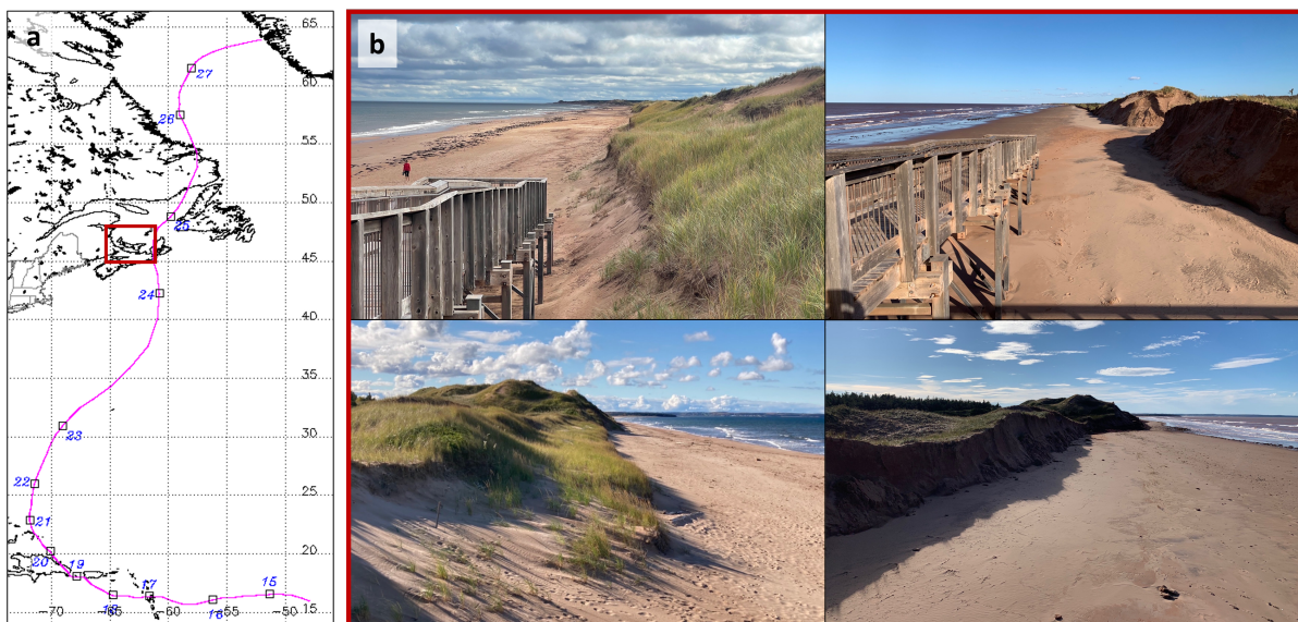
Figure 1.1: (a) Track of Hurricane Fiona following the eastern coast of North America, making landfall in Atlantic Canada (IBTrACS, 2022); (b) Before and after photos showing significant dune erosion on Prince Edward Island, Canada following high storm surge and wave action due to Hurricane Fiona (CoastSnap, 2022).
