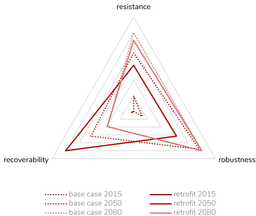
Figure 44: Thermal resilience indices performance of retrofit proposal (solid line) compared to base case (dotted line) in 2015 (dark red), 2050 (red) and 2080 (light red) source: own
