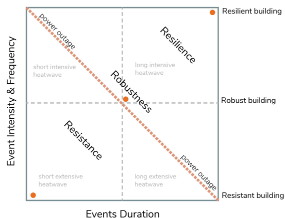
Figure 5: The relation of a heat wave's duration and intensity to a resistant, robust, and resilient building's response. The plot surface area is divided into categories of "short/long" and "intensive/extensive" heat waves, with power outages occurring in "short-intensive" and "long-extensive" heat wave scenarios. Orange dots are positioned to represent the assumed intensity and frequency that the corresponding building design can withstand. adapted from: Attia et al., 2021, p. 6
