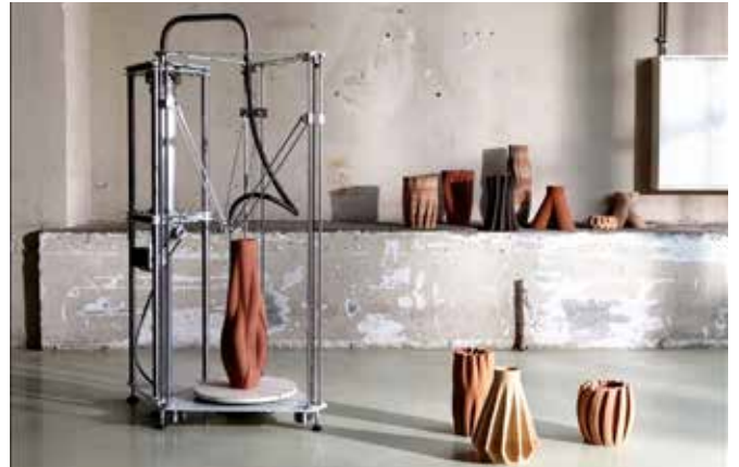
Ceramic-porcelain-3d-printer by Olivier van Herpt Logo https://oliviervanherpt.com/blue-and-white-porcelain/
