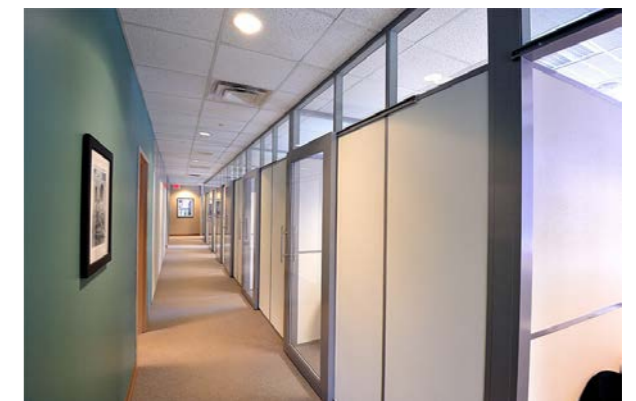
Fig. 9.4 NxtWall (2018) Flexible office wall system BUILDING LAYERS | 89
