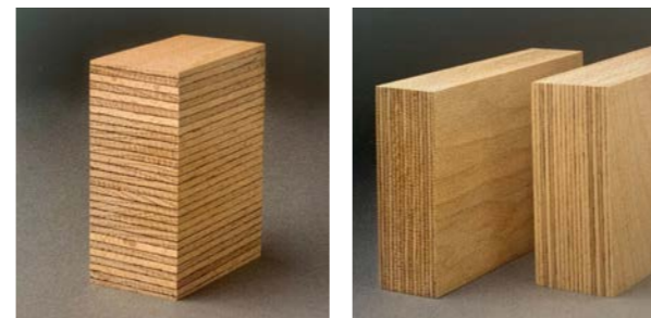
Fig. 6.9 Merz, Niemann, & Torno (2021) Beech LVL with transverse layering (left) and edgewise vertical layering (right)
