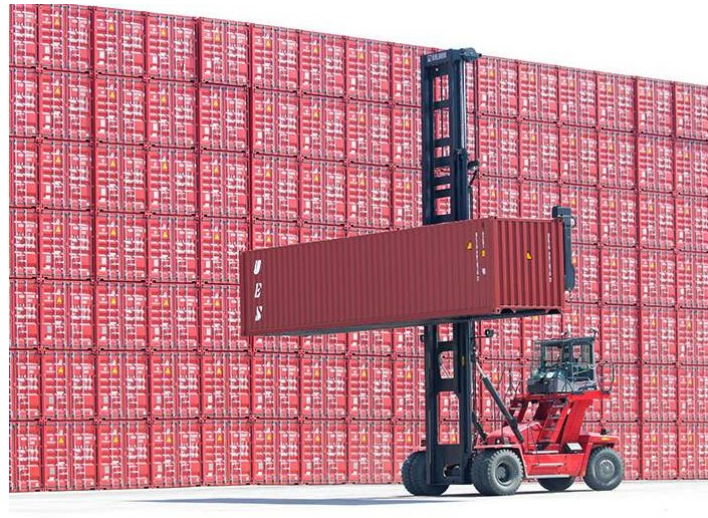
Figure A-5: Empty handler with a 40-foot empty container in front of an empty stack
