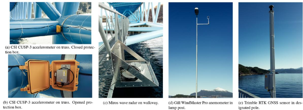
Figure A.3: Measurement equipment used at the Bergsøysund bridge (Kvåle and Øiseth, 2017).
