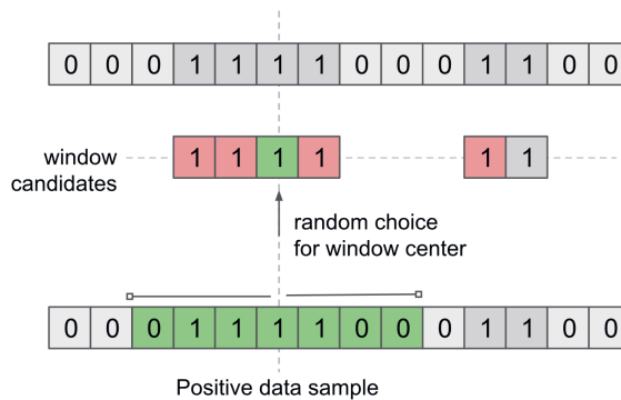
Figure 7.5: Illustration of the process used to select positive laughter samples for our machine learning tasks. Given the binary laughter / non-laughter annotations for a particular segment, we select a location for the window center from the positively-annotated intervals in the signal. We then extract a window of 1.5 seconds around the chosen center. We pad if necessary.
