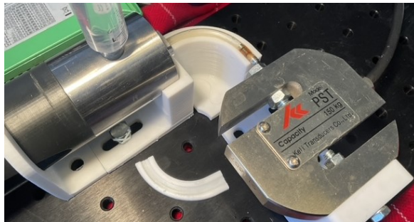
Figure E.6: Close up showing the 90 degrees curvature tube holder module. The white part next to the tube holder module is the top part of the tube holder module, used for securing the tube in place so no movement occurs from the tube itself. This is used so the wave can travel through the tube without losing additional energy to unwanted movement of the tube.
