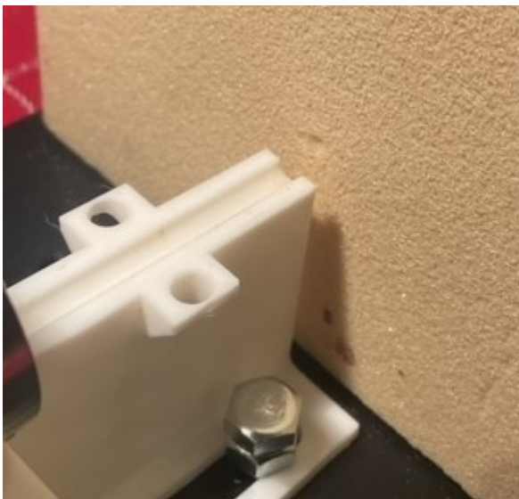
Figure 5.5: Small indentation observed after striking the same spot for 30 repetitive strikes with a compression distance of the spring of 40 mm. (Tube is removed in order to see the indentation better from an angle)
