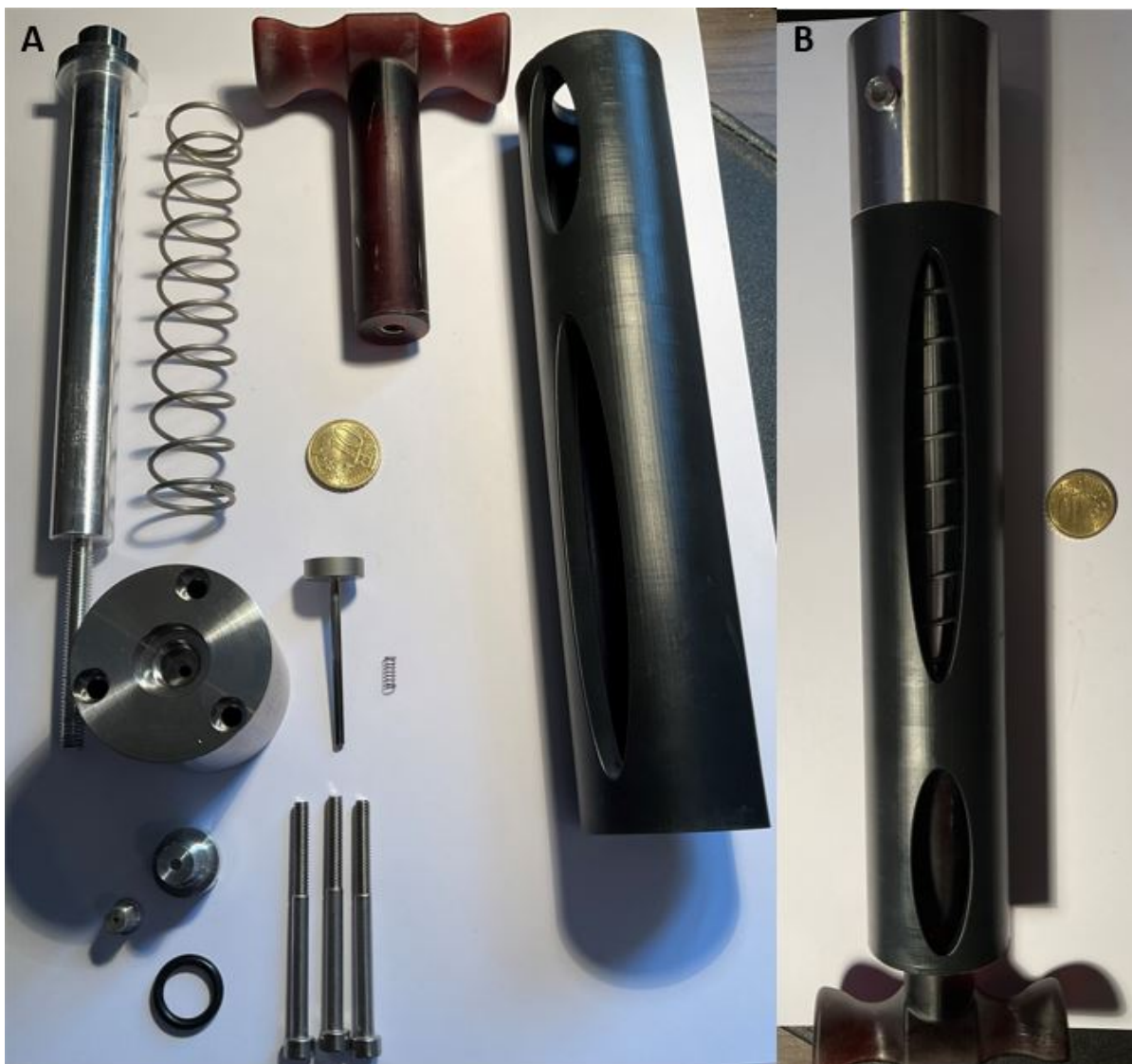
Figure 4.11: Fabricated end product of the proof-of-principle prototype impulse generator part with A) an exploded view, with the components disassembled, and B) a view of the pieces assembled.
