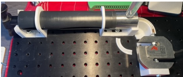
Figure E.2: Proof of principle experiment with the 90 degrees curvature tube holder module. This setup was utilized in order to proof that the instrument would still have an impact output if the tube was bend at a 90 degrees angle over the entire length of the tube excluding the tip part.
