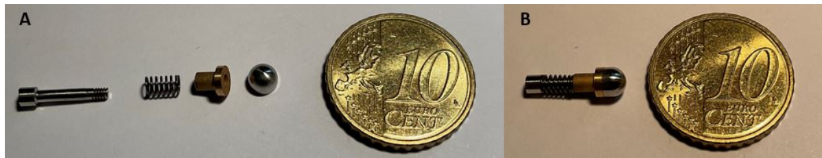
Figure 4.10: Fabricated end product of the proof-of-principle prototype working head part with A) an exploded view, with the components disassembled, and B) a view of the pieces assembled.
