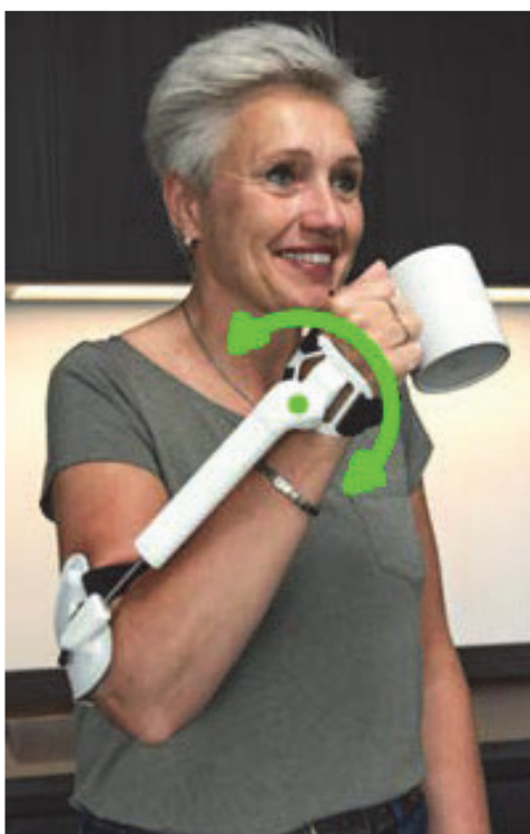
image / figure 2: Current version in use, green arrows indicating wrist abduction/adduction
