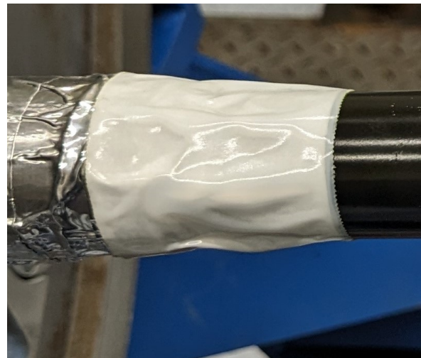
(b) Thermocouple protected from flow using tape.
