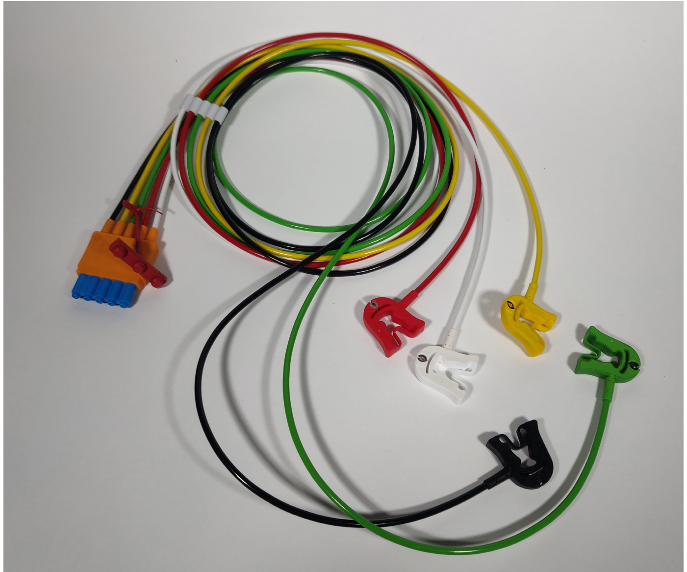
Figure 3: An ECG Lead set
