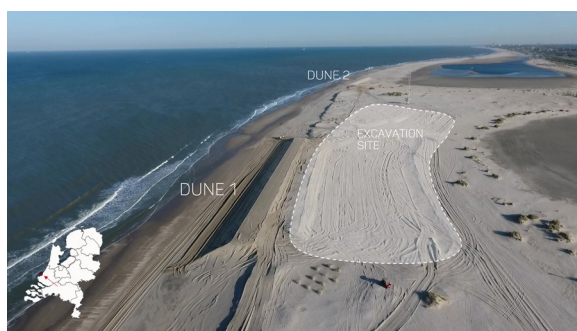
Fig. 2 Aerial view of the field site including Dune 1, Dune 2, and the excavation site from which sediment was excavated for the construction of both dunes. The field site location within the Netherlands is displayed on the inset map.
