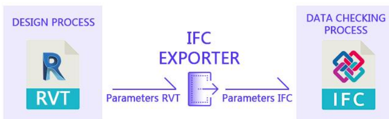
Figure 6: IFC Exporter position between design and data checking process (own illustration)
