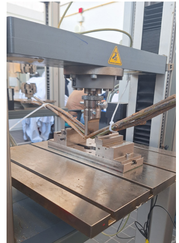
Figure 63: Salix Babylonica bundled bending test
