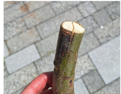
Figure 49: Salix Babylonica I shear failure
