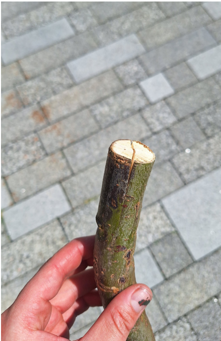
Figure 55: Salix Babylonica I after shear failure
