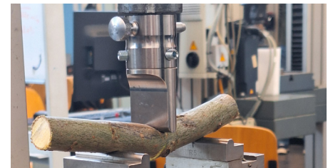
Figure 50: Salix Caprea II during bending
