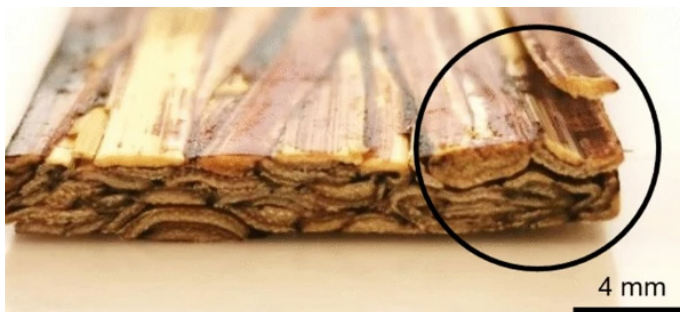
Figure 18: Beam made from reed with adhesion problem Albrecht et al., 2023
