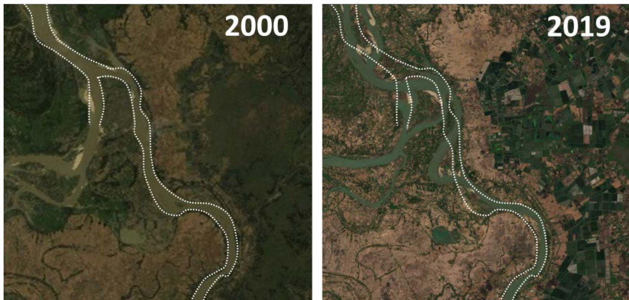
Figure 2.56: Morphology of the Myitmaka River at different points in time: where to locate a port? (left: Landsat 4-5 TM L2 image courtesy of the U.S. Geological Survey processed by Sentinel Hub is licenced under CC BY; right: ‘Copernicus Sentinel data 2019’ for Sentinel data is licenced under CC BY).
