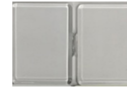
Figure 5.22: PC before (left) and after (right) exposure to UV-C (Covestro, 2021).
