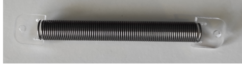
Figure A.7: Spring attached to two mounts for tensile testing
