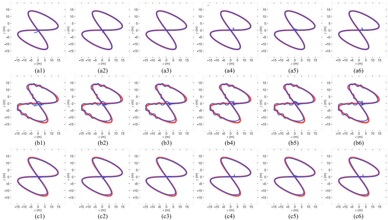
Fig. 7. Simulation results of the eight-type trajectory. Top: Tracking control of a CMR using the nominal controller in Lemma 1. Middle: Tracking control of a CMR under false data injection attacks designed by Algorithm 1. Bottom: Tracking control of a CMR under the secure controller learned using Algorithm 2.
