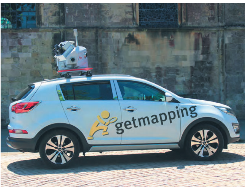
▲ Figure 1: All sensors of the Pegasus:Two Ultimate are rigidly integrated in the same casing; the rack can be mounted on a variety of vehicles including cars (left).
