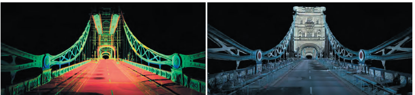
▲ Figure 3: Laser point cloud of Tower Bridge in London, intensity coloured (left) and the point cloud resulting from colourizing from simultaneously captured 360-degree panoramic images.
