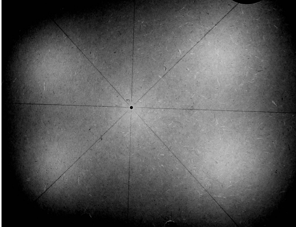
Figure 3.6: Photograph of multiple illuminance peaks on the measurement surface, as seen with luminaires D_1 and E_1 when using the large light field setting of the luminaire. Just visible are the 4 measurement lines drawn at the lighted surface. Note that the centres of the illuminance peaks lie next to these lines.
