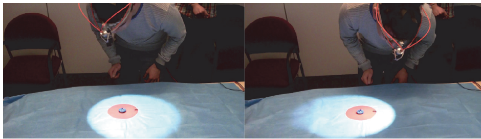
Figure A.3 Demonstration of the functionality of the steerable head-mounted light, when moving the head to the right of the wound (left picture) and to the left of the wound (right picture).
