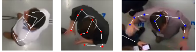
Figure 2: Different gesture ranges of body key-points (no gesture, normal gesture - red, wide gesture - blue)
