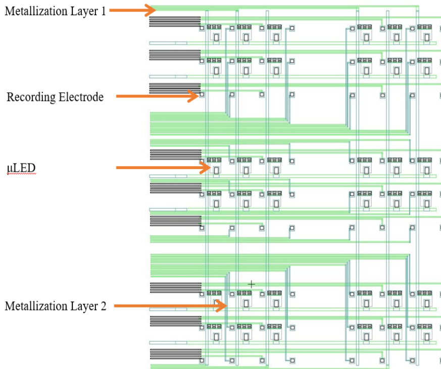
Figure 3.6: Optogenetic array with two metallization layers separated by a dielectric
