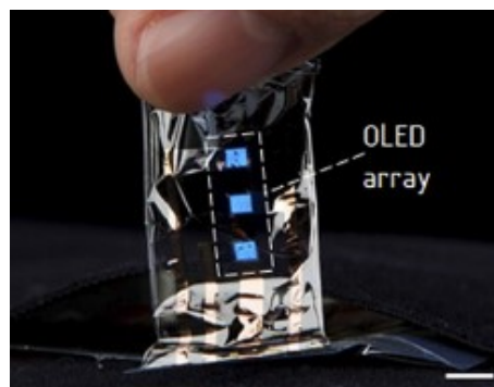
Figure 2.5: OLED array on a parylene-c substrate of 2 \mu\text{m} thickness [23]
