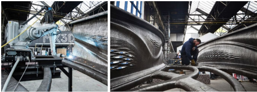
Fig. 4.1 Robotic fabrication of the metal MX3D bridge (2021)
