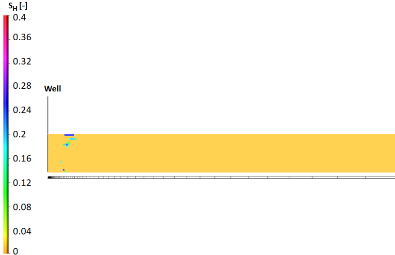
Figure 4.62: 2D plot for hydrate saturation after 5 years of injection, case study Reservoir A, CO 2 injection at 12°C (275.15K).
