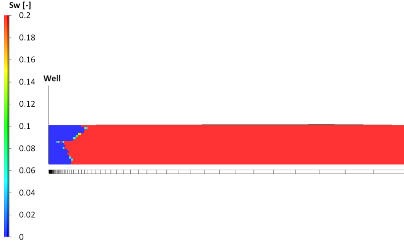
Figure 4.53: 2D plot for water saturation after 5 years of injection, case study Reservoir A, CO 2 injection at -5°C (268.15K).
