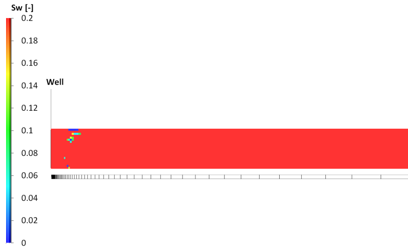
Figure 4.63: 2D plot for water saturation after 5 years of injection, case study Reservoir A, CO 2 injection at 12°C (275.15K).
