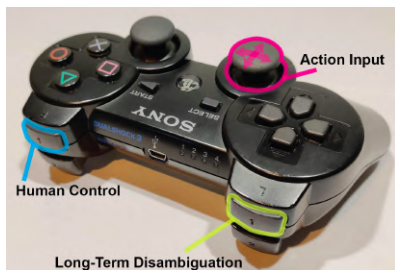
Fig. 3: Teleoperation device for giving continuous action feedback. For safety reasons, the user can give corrections only if the blue button is kept pressed. The green one is used for activating the long-term disambiguation as described in Sec. III-B.
