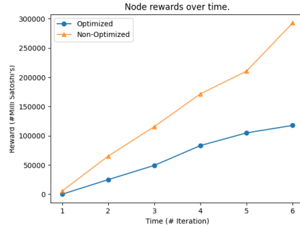
(f) Figure depicting the reward obtained when network optimization is not performed and is performed (baseline) using placement strategy: k means and transaction amount: 10000
