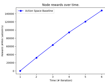
(a) Figure depicting the channel placement reward obtained using placement strategy: fee weighted centrality and transaction amount: 10000
